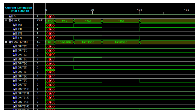
Fig. 6: Conventional 4 to 16 Decoder
