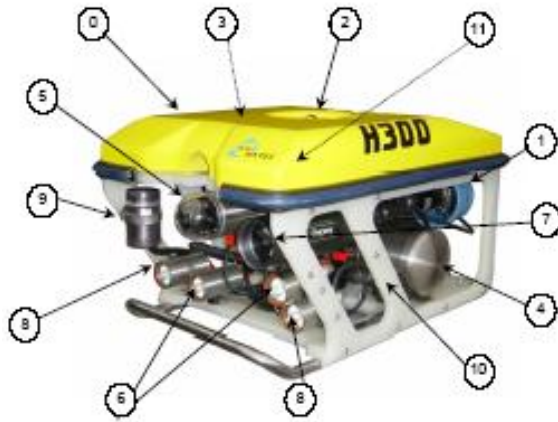
Fig.3.1: ROV System (Vehicle) parts shown with number markings without & with CECH300 clear water cylinder.
