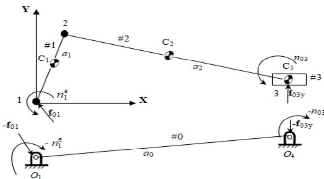
Fig. 1 Definitions of parameters for a planar slider-crank mechanism
