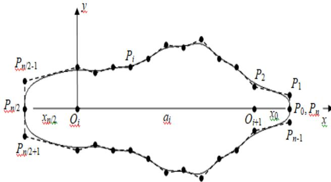
Fig. 3 Closed cubic B-spline curve representing link shape and its control points
