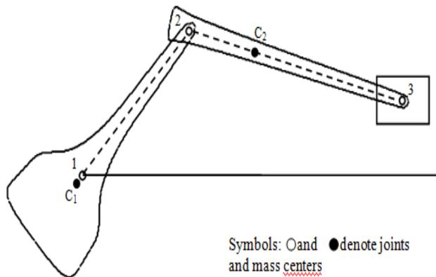
Fig. 8 Optimized link shapes for planar slider-crank mechanism [figure drawn on scale]
