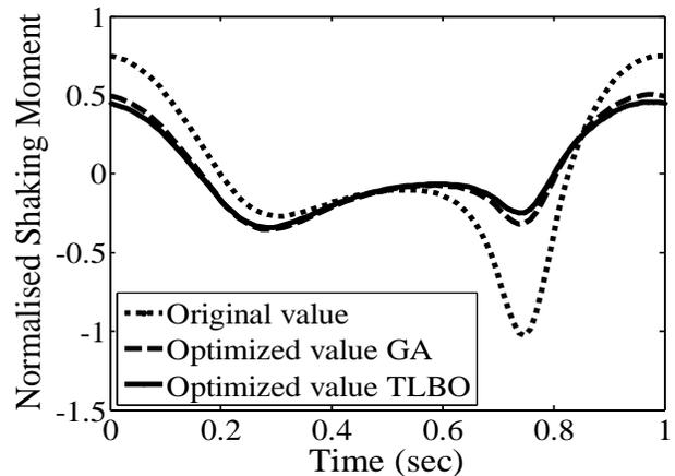
Fig. 7 Variations of shaking force and shaking moment for complete crank cycle
