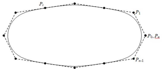
Fig. 2 Closed cubic B-spline curve and its control points
