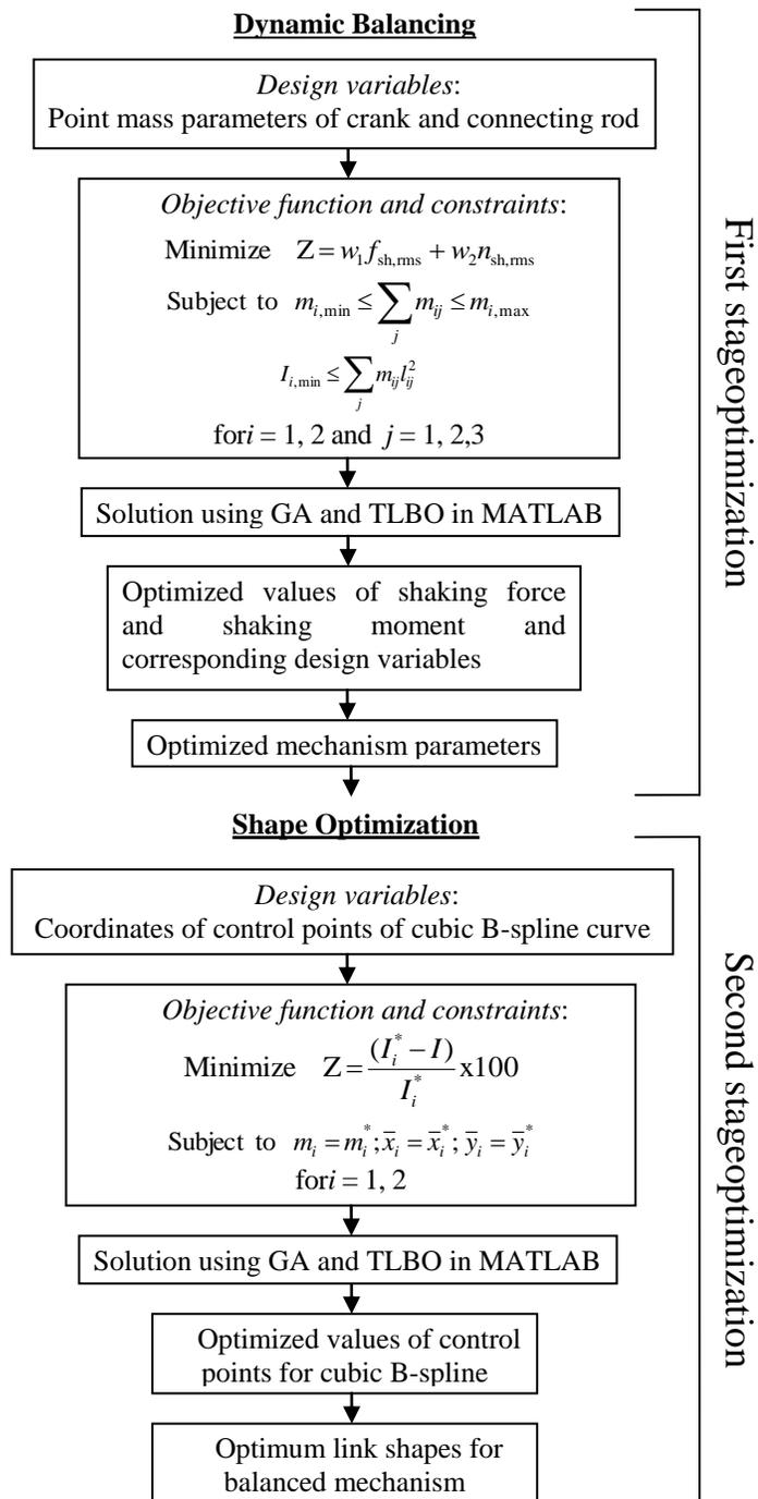
Fig. 4 Two stage optimization scheme to balance mechanism and shape synthesis
