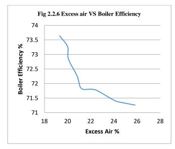
It is found from the above iterations is that the excess air varies directly with the losses in the boiler and inversely with the efficiency of the boiler. If excess air is increased or decreased correspondingly the efficiency decreases or increases and losses increases or decreases.
