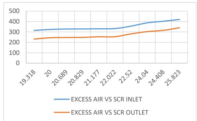
Fig 4.2 Excess Air VS  $NO_x$  at SCR Inlet and Outlet
