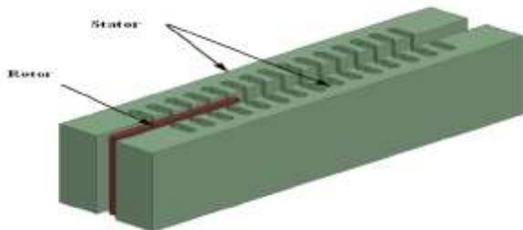
Figure 2: Construction of DSLISM
