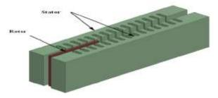
Figure 2: Construction of DSLSM
