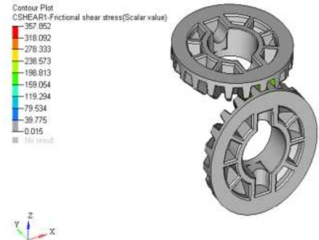
Fig 18. Contact stress distribution of bevel gear after modification
