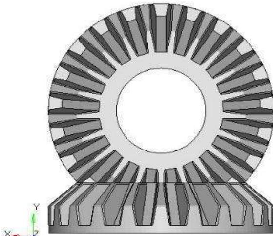
Fig 1. Bevel gear front view
