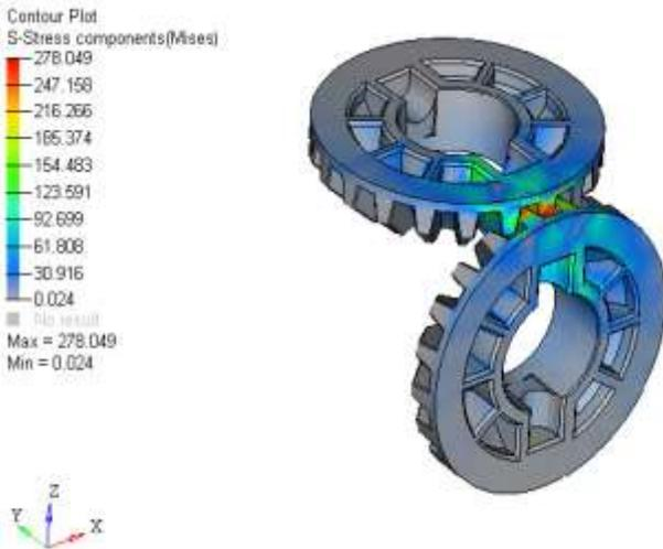
Fig 10. Tooth bending stress distribution before modification.
