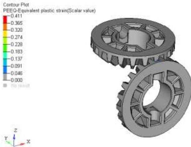
Fig 20. PEEQ of bevel gear after modification
