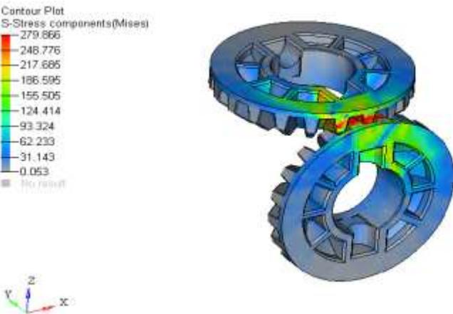
Fig 16. Tooth bending stress distribution of bevel gear after modification
