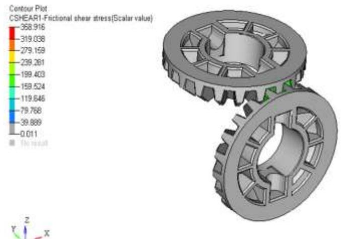
Fig 24. Contact stress distribution of bevel gear after modification
