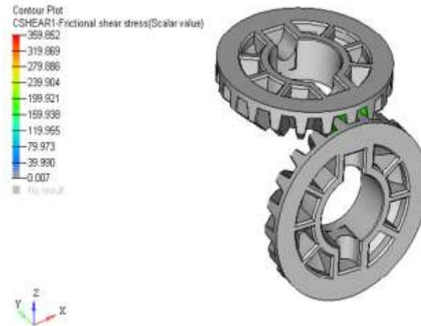
Fig 21. Contact stress distribution of bevel gear after modification
