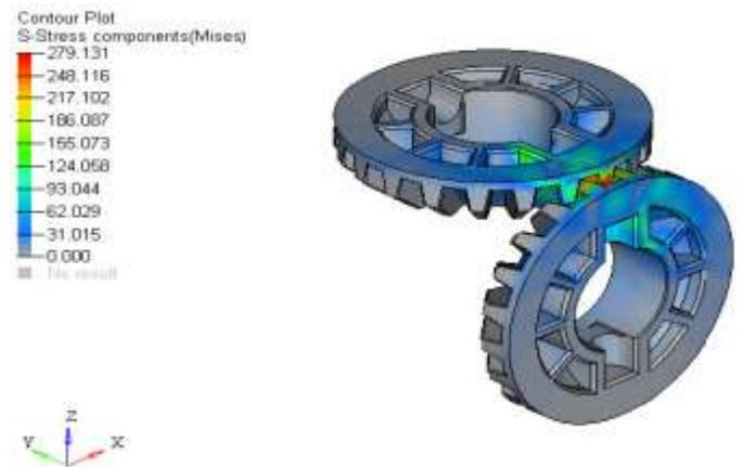
Fig 7. Tooth bending stress distribution before modification.
