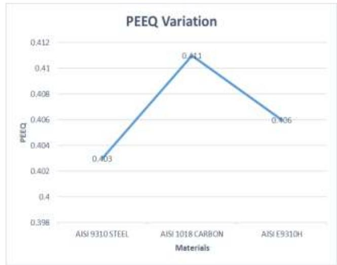
Fig 26. PEEQ variation for modified design
