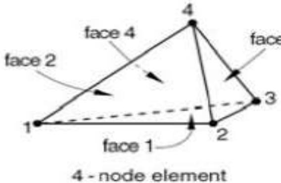
Fig 4. Nodes and face number of the element.
