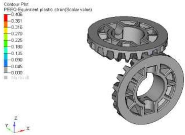
Fig 23. PEEQ of bevel gear after modification
