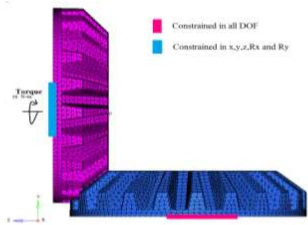
Fig 6. Loading and boundary conditions
