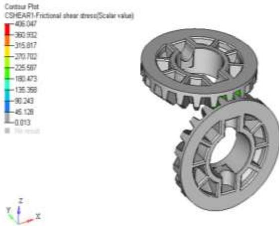
Fig 9. Contact stress before modification
