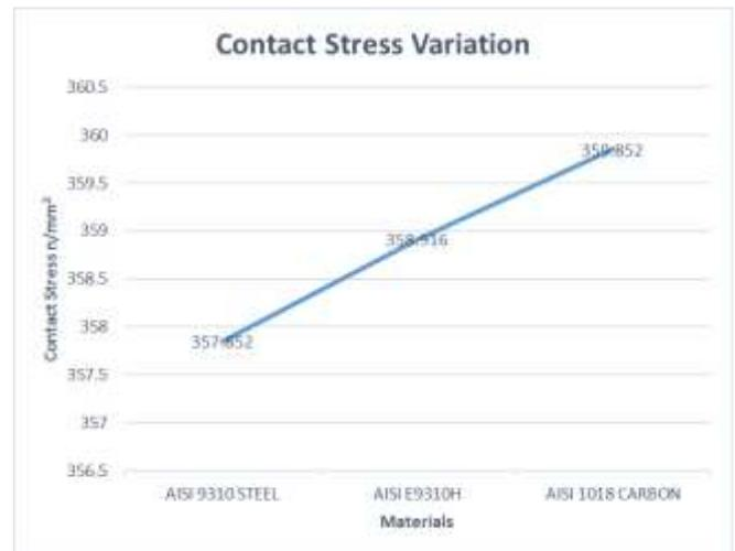
Fig 29. Contact stress variation for modified design.
