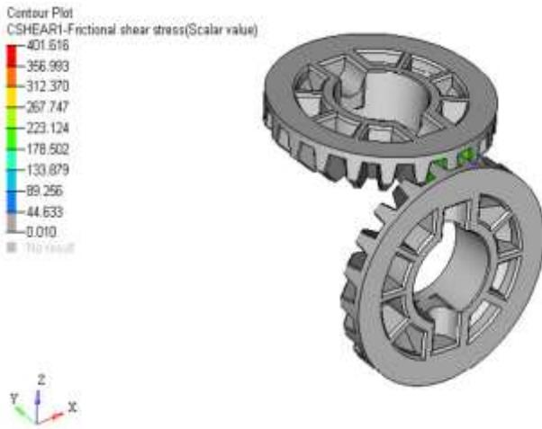
Fig 15. Contact stress before modification
