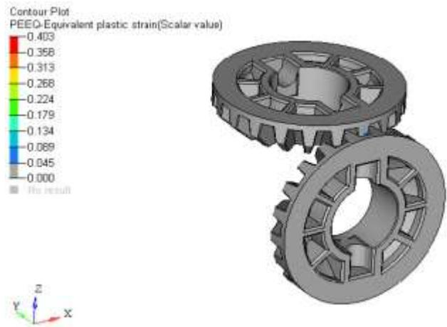
Fig 17. PEEQ of bevel gear after modification
