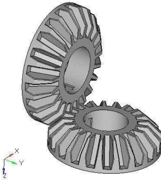
Fig 2. Bevel gear isometric view
