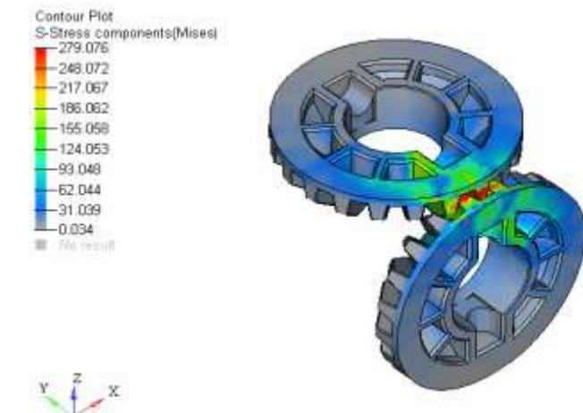
Fig 22. Tooth bending stress distribution of bevel gear after modification
