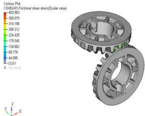
Fig 12. Contact stress before modification
