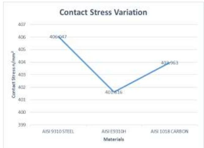
Fig 28. Contact stress variation for base design
