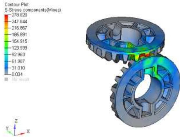
Fig 19. Tooth bending stress distribution of bevel gear after modification
