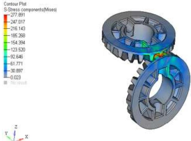
Fig 13. Tooth bending stress distribution before modification.
