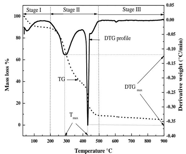
Fig.4. TG and DTG curves from the pyrolysis of *S.foetida* of empty fruit in oxygen atmosphere at a heating rate of 10°C/min
