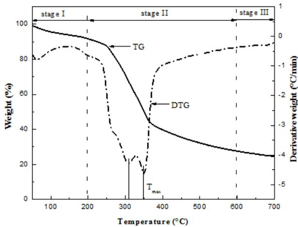
Fig.2. TG and DTG curves from the pyrolysis of *S.foetida* seed in nitrogen atmosphere at a heating rate of 10°C/min
