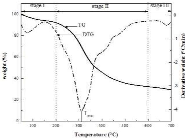
Fig.3. TG and DTG curves from the pyrolysis of *S.foetida* empty fruit in nitrogen atmosphere at a heating rate of 10°C/min
