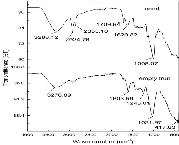
Fig.5.FTIR analysis of *S.foetida* of empty fruit and seed at a heating rate of 10°C/min
