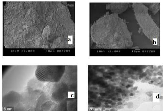
Figure 2 SEM images of Ce<sub>0.4</sub>Zr<sub>0.6</sub> (b and c)TEM images c and d
