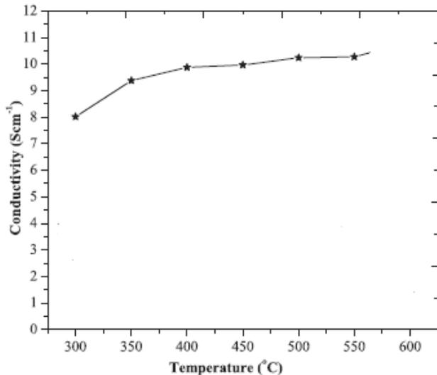
Figure 4: Arrhenius plot of DC conductivities of  $Ce_{0.4}Zr_{0.6}$  in air D.C.
