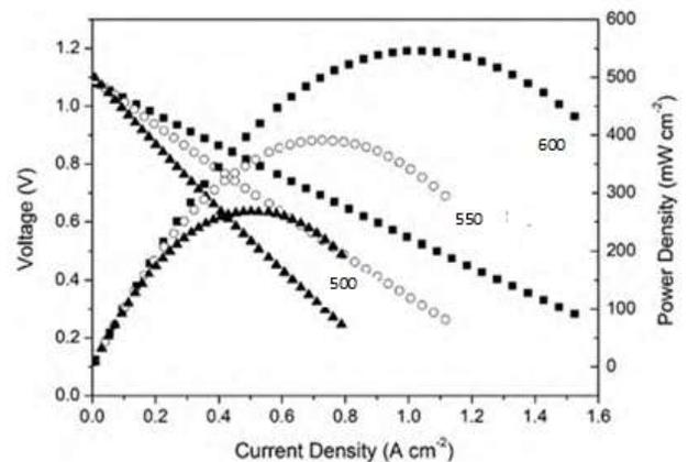
Figure 3 Cell voltage and power density as a function of current density in air in rage of 500-600°C
