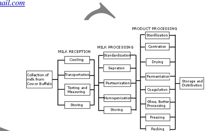
Fig.1- Block diagram of milk processing
