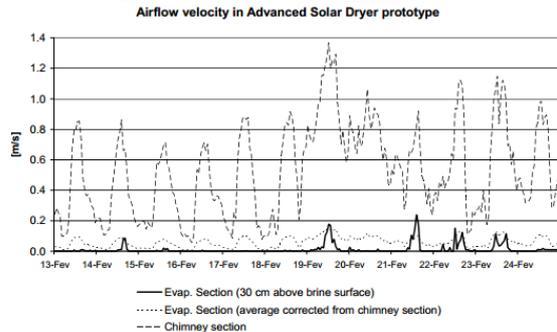
Fig. 4- Approximate Airflow velocity in Solar Dryer section
