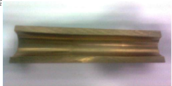
Fig 3. (a) Cut view of brass cavity of 42 GHz 200 kW gyrotron
