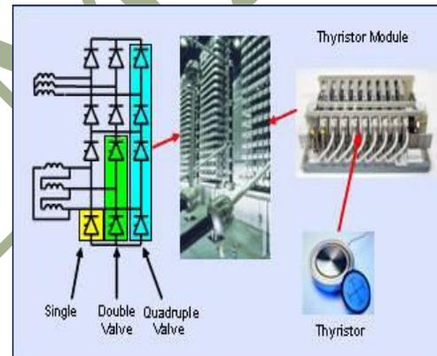
Fig. 4. HVDC thyristor valve arrangement
