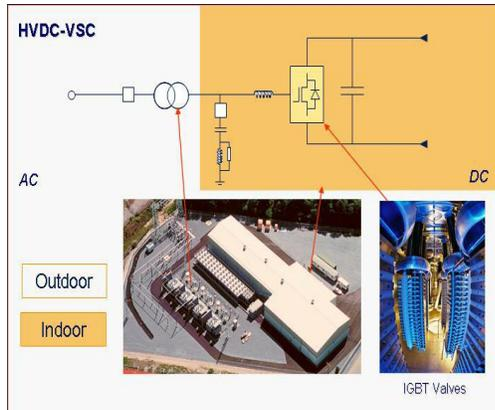
Fig. 3. HVDC with voltage source converters
