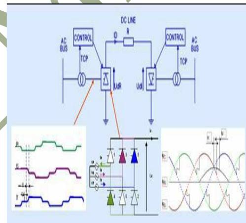
Fig. 6. Control of VSC-based HVDC transmission
