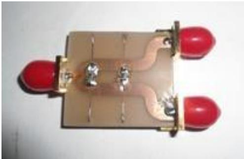
Fig. 2. Photograph of the fabricated Power divider
