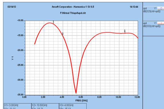
Fig.5 Simulated result of Isolation  $S_{32}$ ,  $S_{23}$
