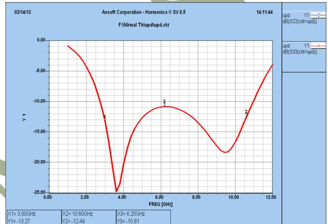
Fig.4 Simulated return loss  $S_{22}$ ,  $S_{33}$
