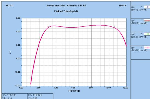
Fig.6 Simulated Insertion loss  $S_{12}$ ,  $S_{13}$ ,  $S_{31}$ ,  $S_{21}$
