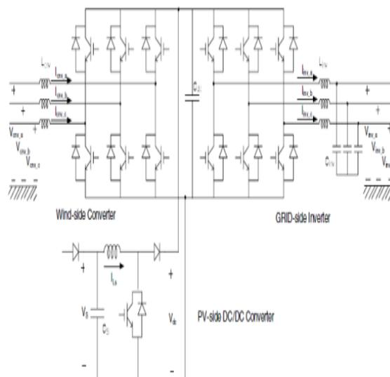
Figure 5 Power electronic interface of the hybrid system
