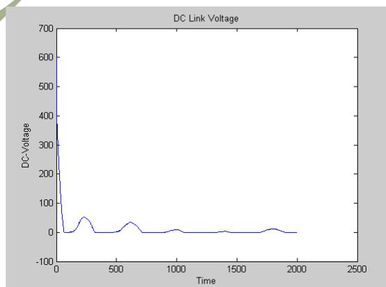
Figure 7 DC Link Voltage
