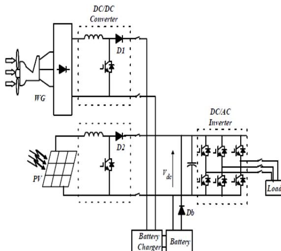
Figure 6 Equivalent circuit of Hybrid PV-Wind System
