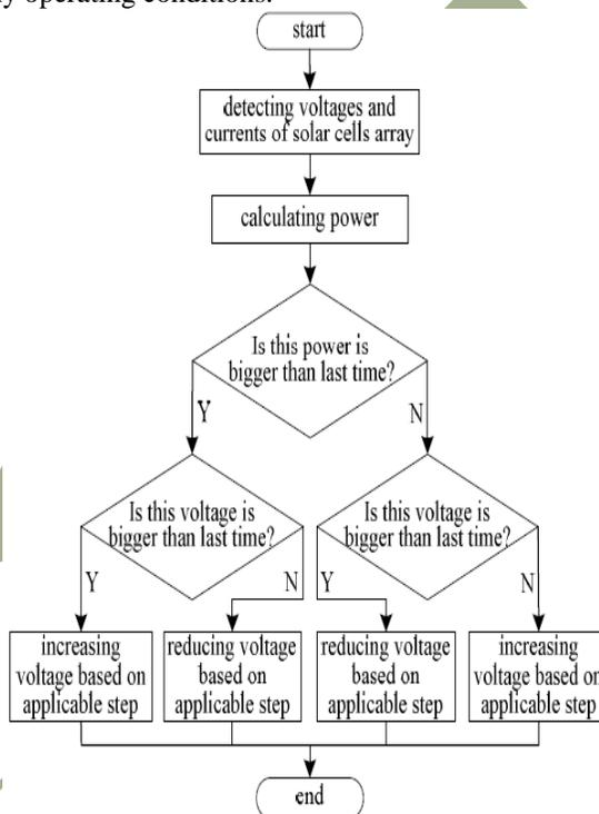
Figure 4. Flow chart of the MPPT technique
