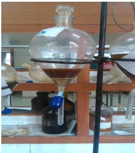
Figure 4: Separate layers of aqueous and organic layers
