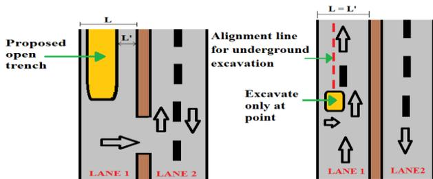
Figure 1. (A) Open trench cut Method
