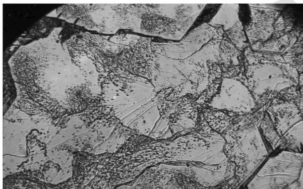
Figure-2: Tiny hillocks observed on the top free surface.
