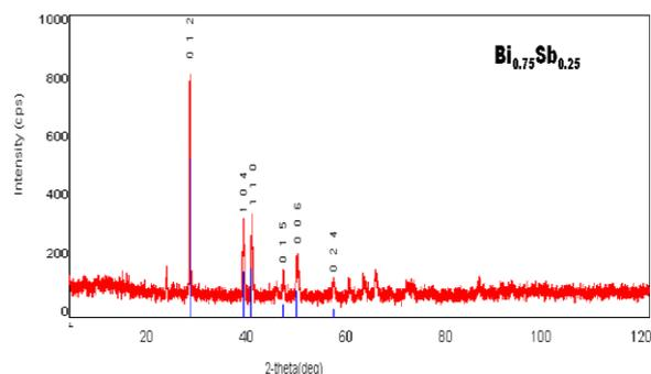
Figure-5: X-Ray diffraction pattern of  $\text{Bi}_{0.75}\text{Sb}_{0.25}$
