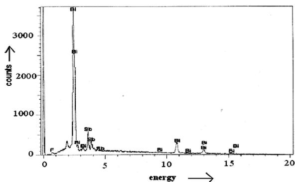
Fig.-6. Compositional analysis's of  $\text{Bi}_{0.75}\text{Sb}_{0.25}$  crystal, by EDAX
