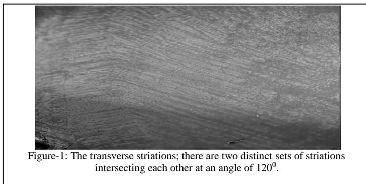
Figure-1: The transverse striations; there are two distinct sets of striations intersecting each other at an angle of  $120^\circ$ .
