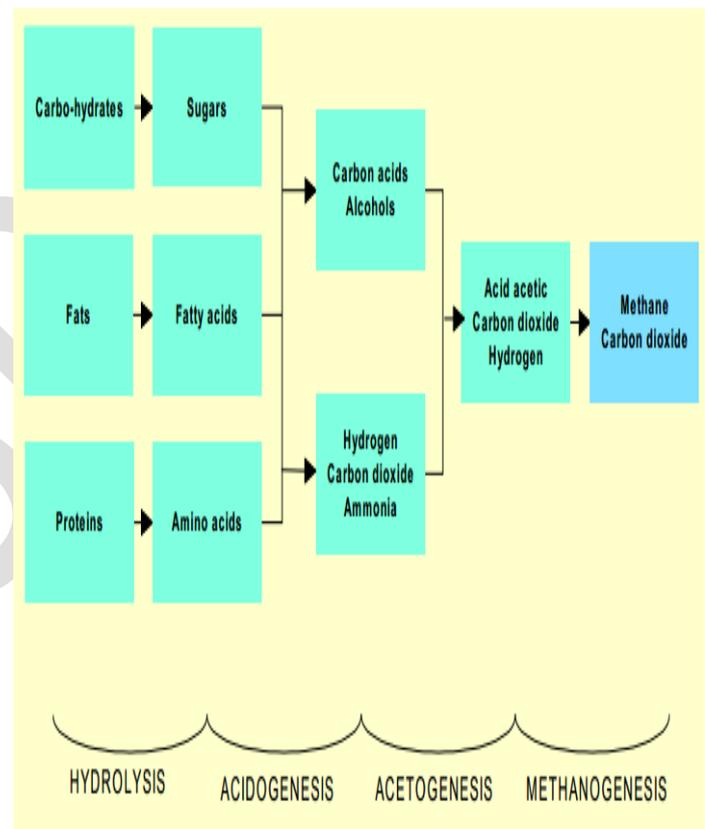
Figure-1. The simplified diagram of the AD process
