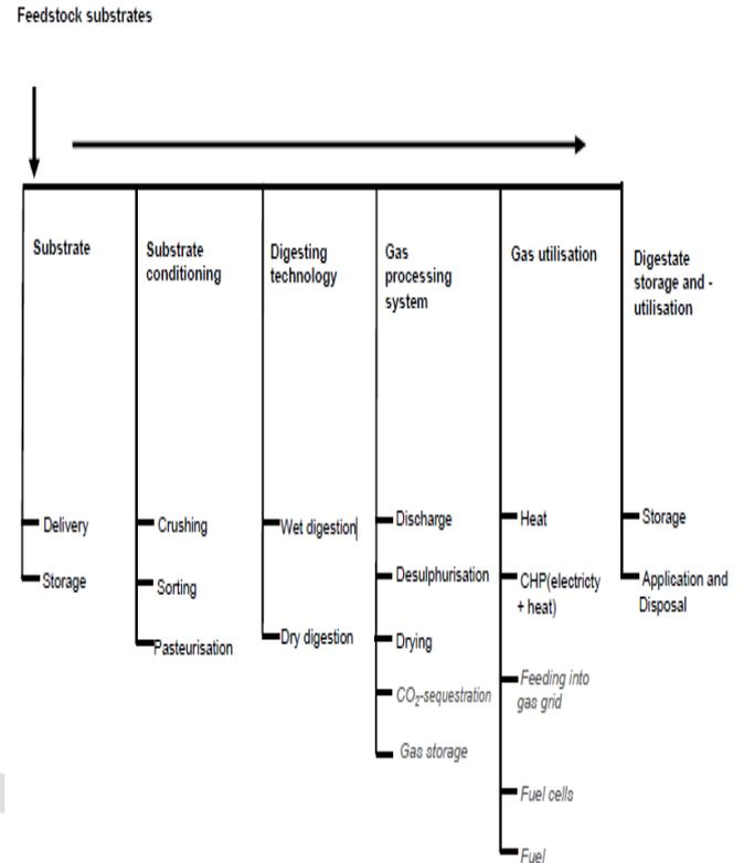
Figure 2. Process steps of biogas technologies
