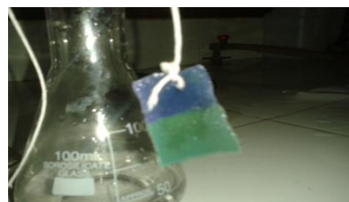
Figure 4. Colour change from green to blue of filter paper when it is dipped in buffer ammonia solution.
