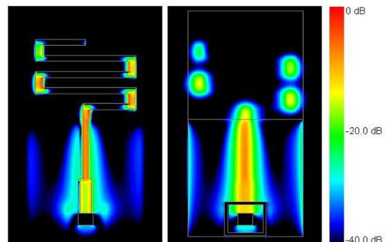
Fig 3.3 Electric Current Magnitude Plot for the MLA.
