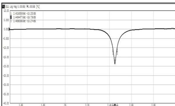
Fig 7.1 S11 Parameters (Return Loss obtained)
