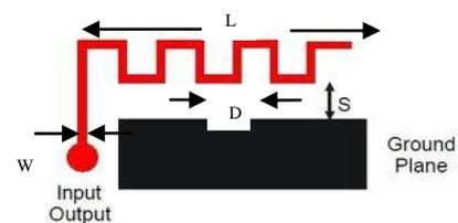
Fig 2.1 Meander Line Antenna
