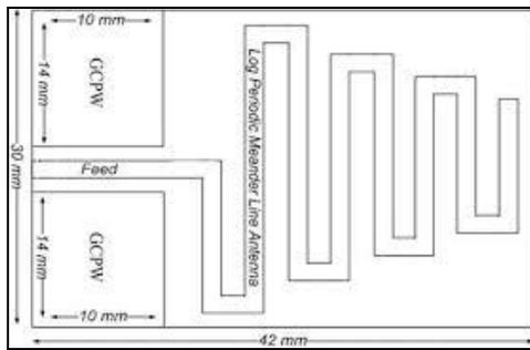
Fig. 5.2 Illustration of Log periodic Meander line antenna.
