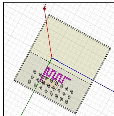
Fig 6.1 HFSS design of MLA with AMC
