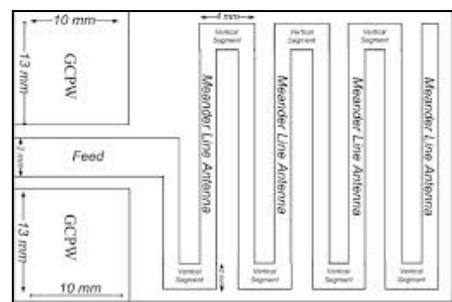
Figure. 5.1 Illustration of MLA with different length of vertical segment.
