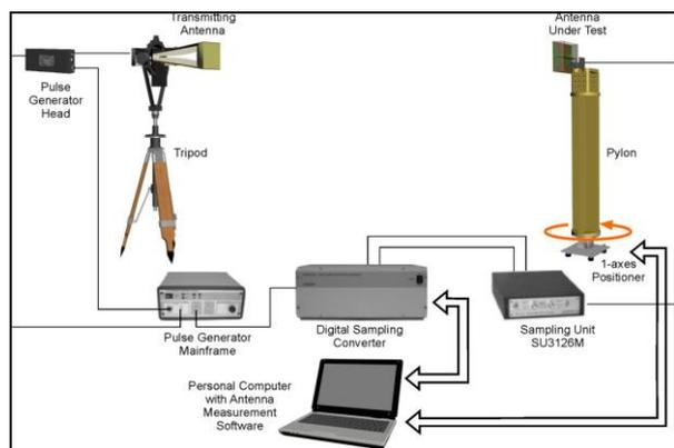
Fig 8.1 Antenna measurement system
