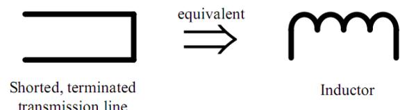
Fig 3.2 Equivalent Model of meander line sections
