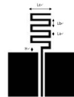
Fig 3.1 Shape of Meander Line Antenna (MLA)
