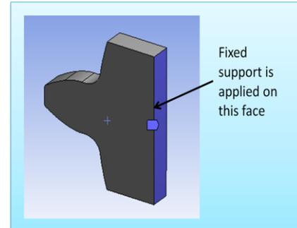
Fig 4 Fixed Support applied
