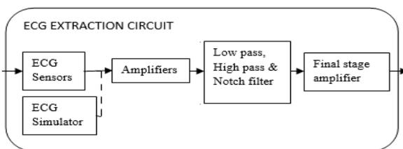
Fig 3. Blocks of ECG extraction circuit
