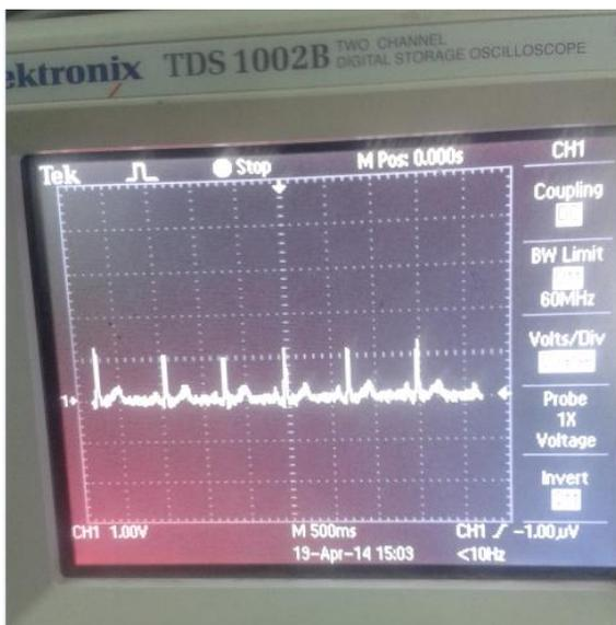
Fig 8.Acquired ECG signal on DSO
