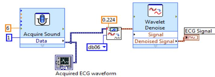
Fig 5. Code for Preprocessing of ECG Signal
