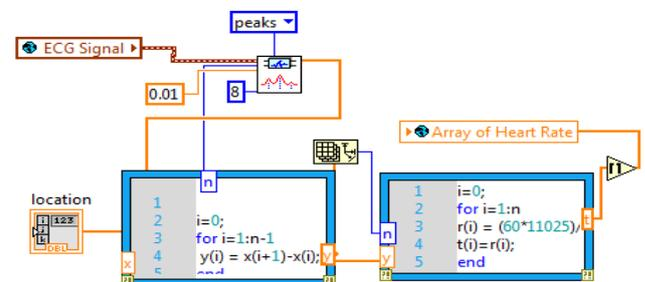
Fig 6. VI for Calculating Heart Rate
