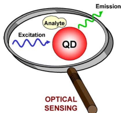
The hybrid sensor consists of anti-TNT specific antibody fragments attached to a hydrophilic QD via metal-affinity coordination. A dye-labeled TNT analogue prebound in
