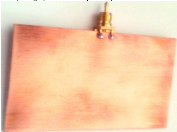
Figure 9. (a)Ground plane of the Fabricated MPA
