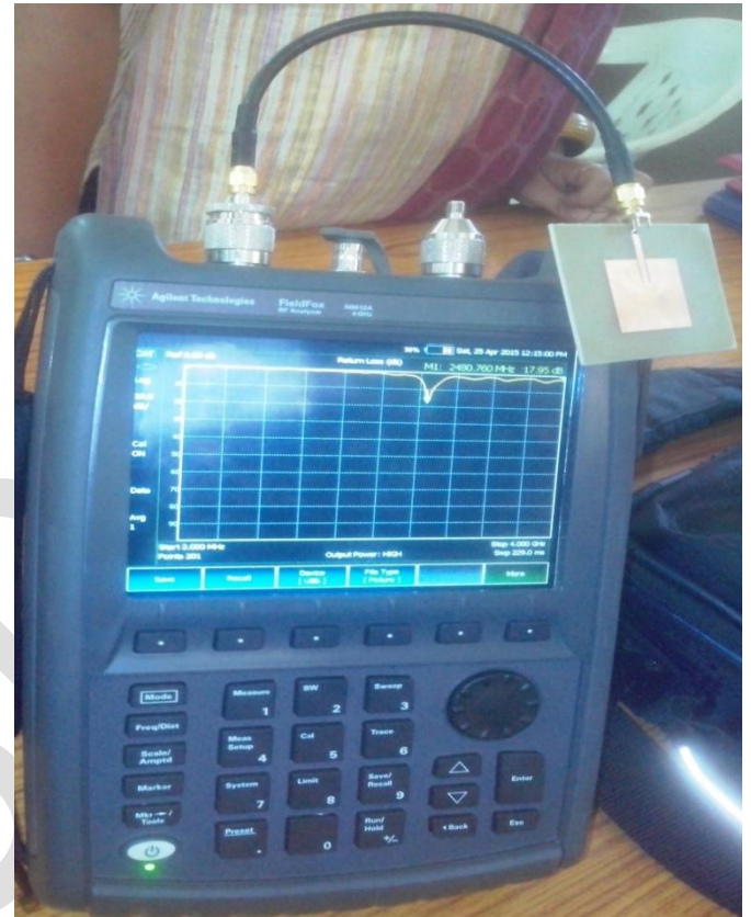
Figure 10 The Set up for the testing of Fabricated MPA
