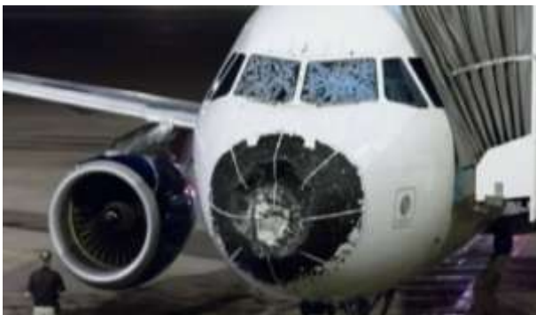
Fig 4B – Aircraft damage due to hail.
