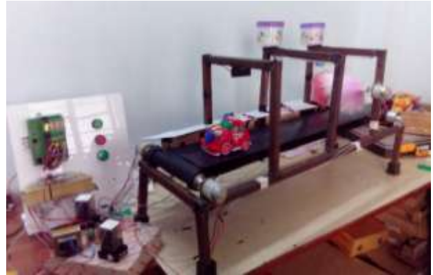
Fig. 9. Prototype Model of PLC Based Car Wash System
