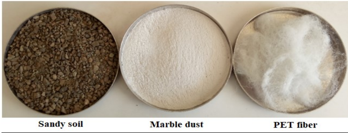
Fig. 1. Photos of sandy soil, marble dust and PET fiber
