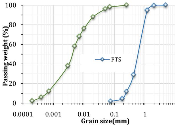
Fig. 1. The grain-size distributions of the expansive and PTS
