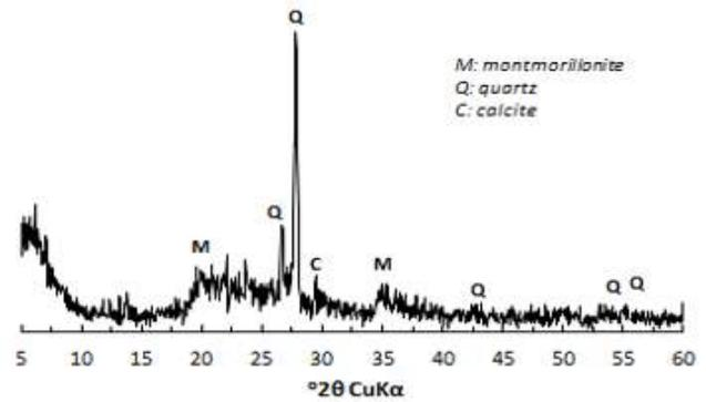
Fig. 2. XRD pattern of the expansive soil
