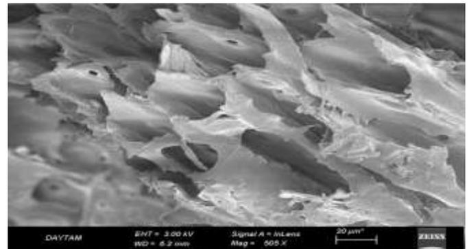
Fig. 3. The SEM image of PTS waste material
