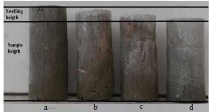
Fig. 4. The change in swelling amounts of the tested samples; a: MIX0, b: MIX1, c: MIX2 and d: MIX3
