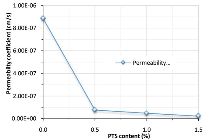
Fig. 5. The change in the permeability coefficients of the tested samples
