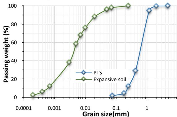
Fig. 1. The grain-size distributions of the expansive and PTS
