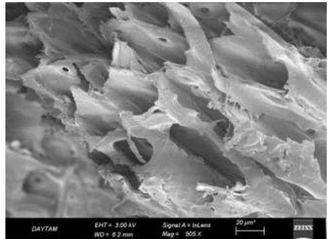
Fig. 2. The SEM image of PTS waste material
