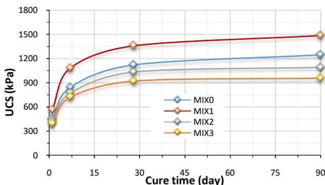
Fig. 3. The change in the UCS value with curing time before freeze-thaw cycles
