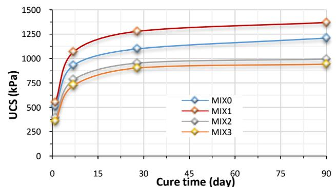
Fig. 4. The change in the UCS value with curing time after freeze-thaw cycles
