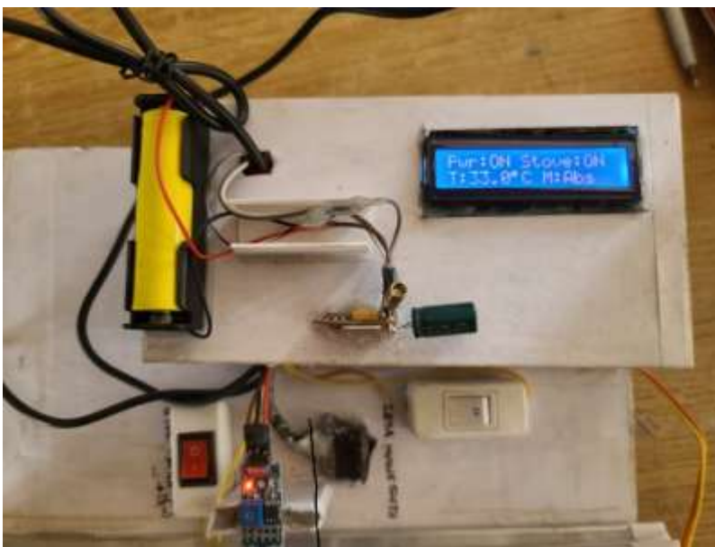
Figure 4. Hardware enclosure layout showing integrated control unit, 16x2 LCD telemetry display (temperature 33.0°C and PIR motion status), switches, and sensor wiring
