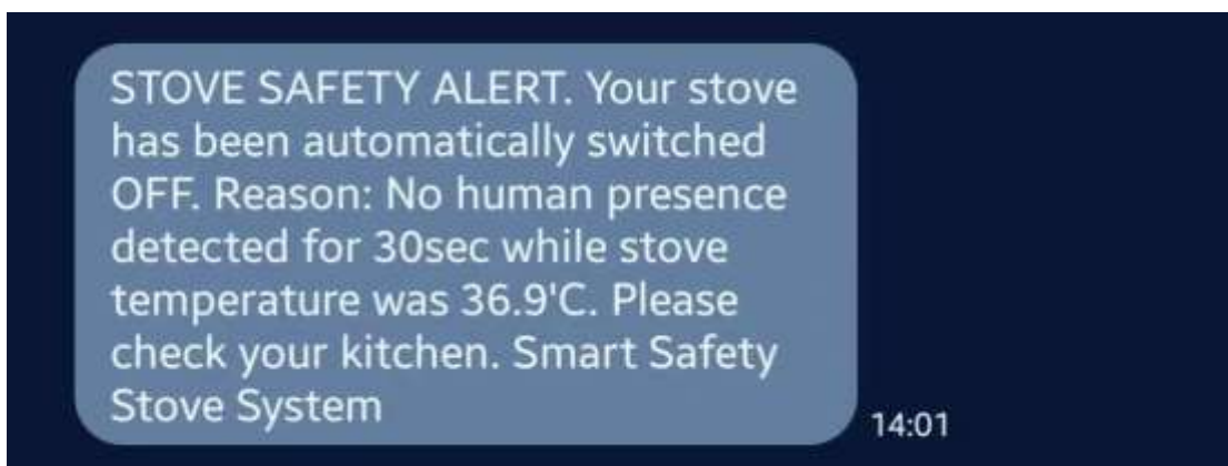
Figure 6. Automated emergency warning SMS dispatched to user upon detecting unmonitored cooking and triggering power isolation.
