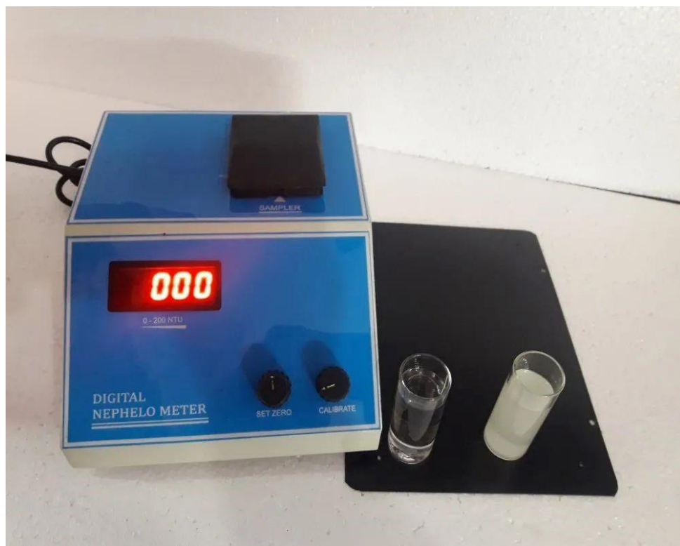
Figure 1: Digital Nephelometer (0-200 NTU range) — used for Turbidity and Sulphate measurements
