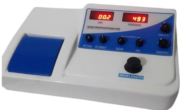
Figure 4: Spectrophotometer — used for Iron, Fluoride, and Nitrate analysis
