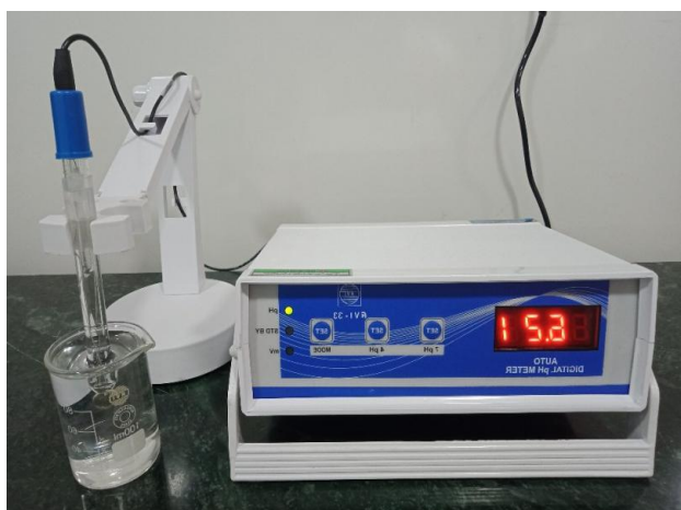
Figure 3: Auto Digital pH Meter (RVI-33) — used for pH measurement
