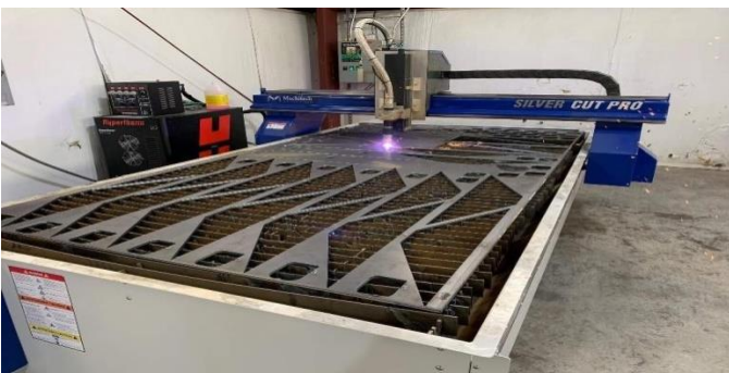
Fig 2.1 A CNC mechanized plasma cutting machine
