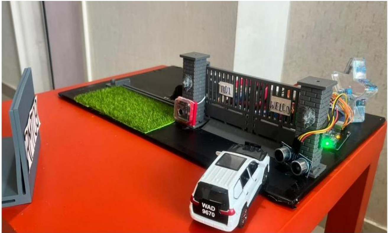
Fig. 3. Deployed physical prototype: Raspberry Pi 5, IMX219 camera, HC-SR04 sensor, and 3D-printed boom-gate assembly.
