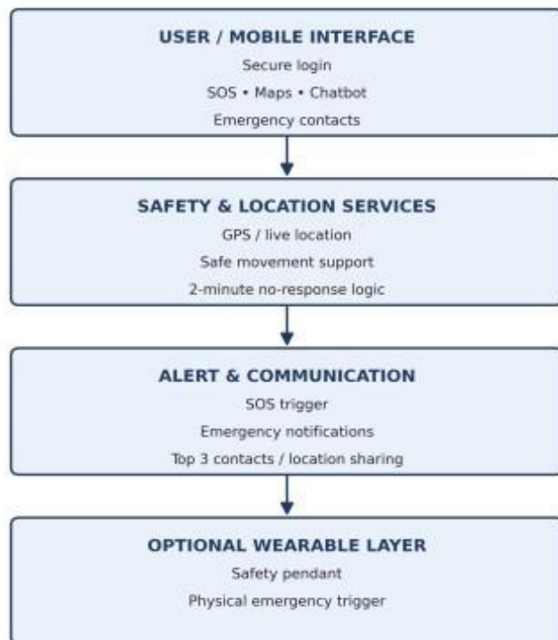
Fig. 2. Proposed SheShield system architecture
