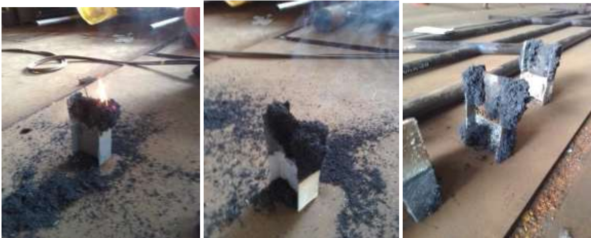
Figure 16: (a/b/c/d) I-Beams during direct fire exposure testing.
