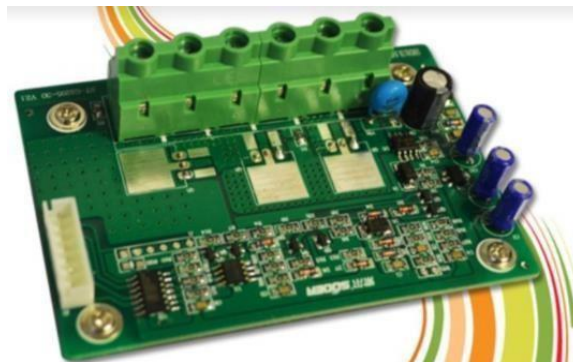
Figure 10 Main Board of Solar Charge Controller
