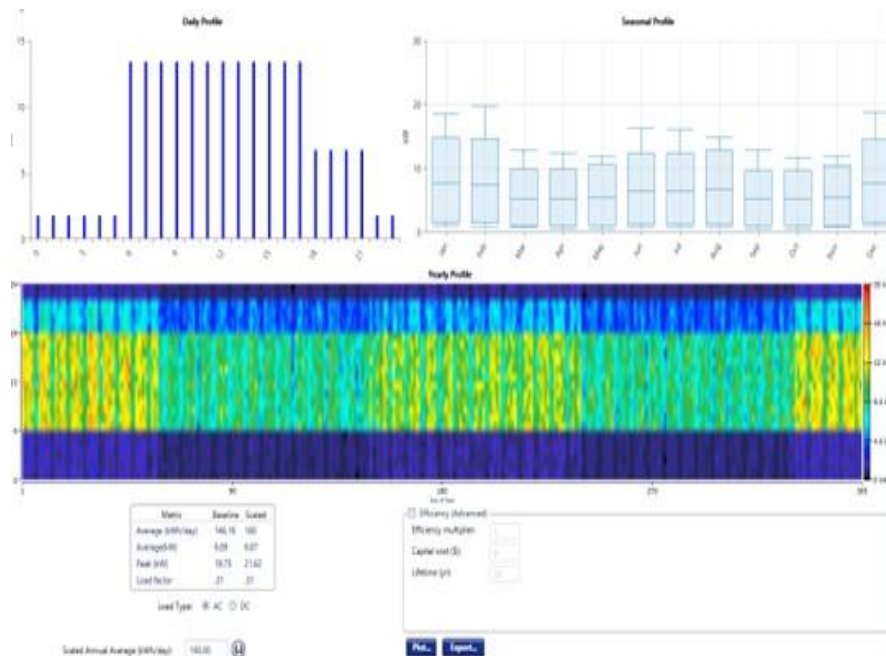
Figure 4.5: Load Profile Overview. This figure shows daily, seasonal, and yearly load profiles of electricity data, along with key metrics such as average energy consumption, average power, peak power, and load factor.
