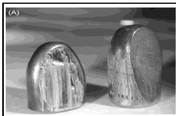
Fig. 3.1 (A) One-sided flattening of bullets after ricochet off glass (Vermeij et al., 2012)
