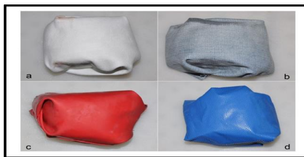
Fig. 3.4 Arrangement of bullets coated with four different common fabrics (a cotton, b jeans, c leather, d nylon) ( Giraud et al., 2016 )
