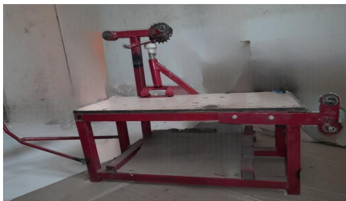
Fig.6.1 Mild Steel Support Frame
