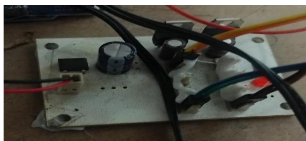
Fig5.19: 5v regulated power supply using 7805 with transformer and Bridge Rectifier
