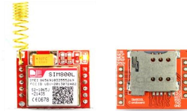
Figure 4: SIM 800L GSM/GPRS Module
