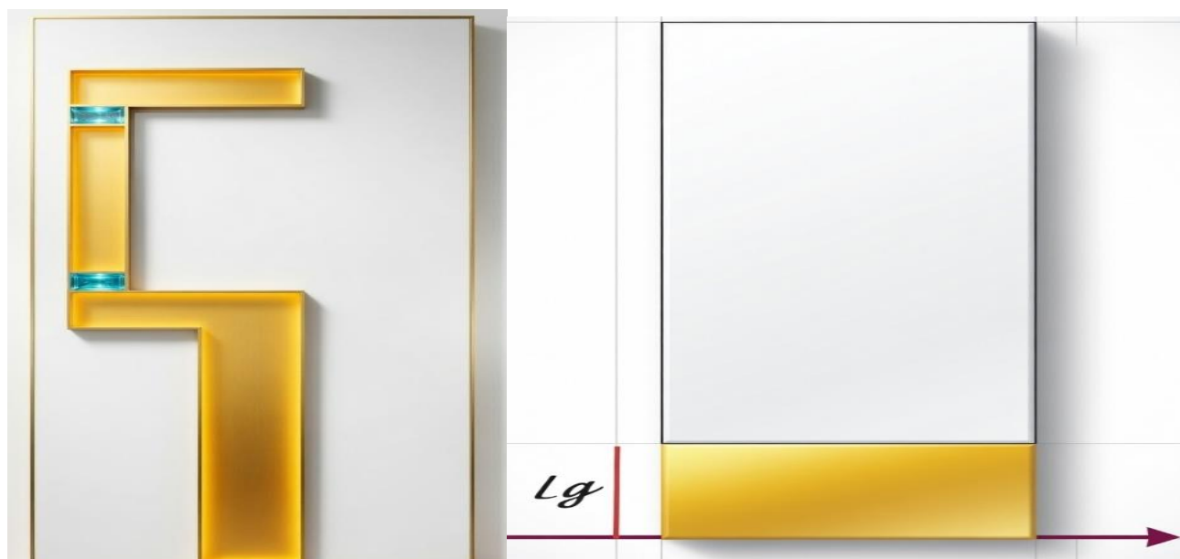
Fig 2: (a) Front view of the antenna with slot, (b) Back view of the Antenna
