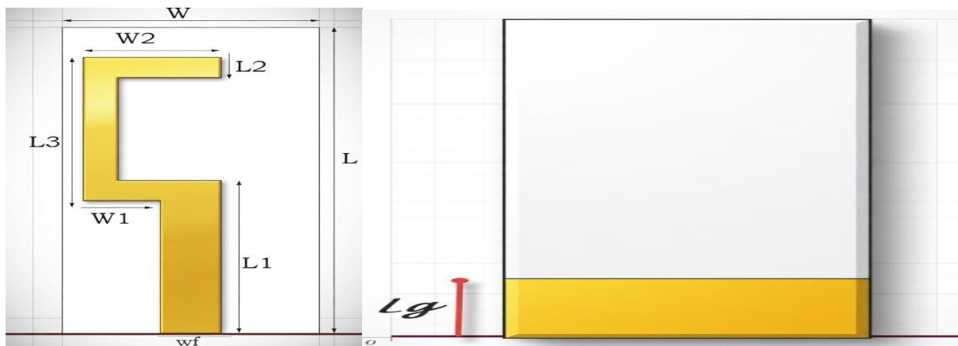
Fig 1: (a) Front view of the antenna, (b) Back view of the Antenna
