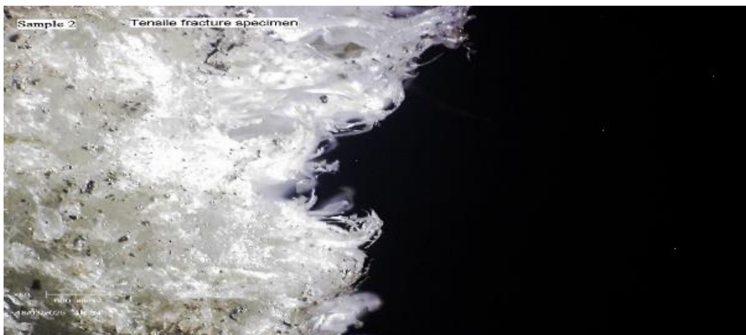
Fig.3.5: Tensile Fracture Surface Micrograph of Sample 2.
