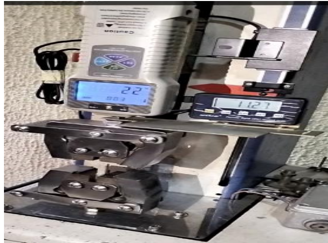
Plate 3.3a: Dumb bell ready for Mechanical Characterization. Plate 3.3b: Tensile Testing Machine.
