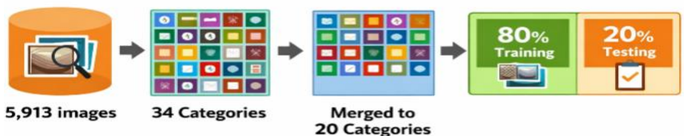
Figure 3: Dataset consolidation and train–test split” showing 5,913 images → 34 categories → merged to 20 categories → 80% training / 20% testing.
