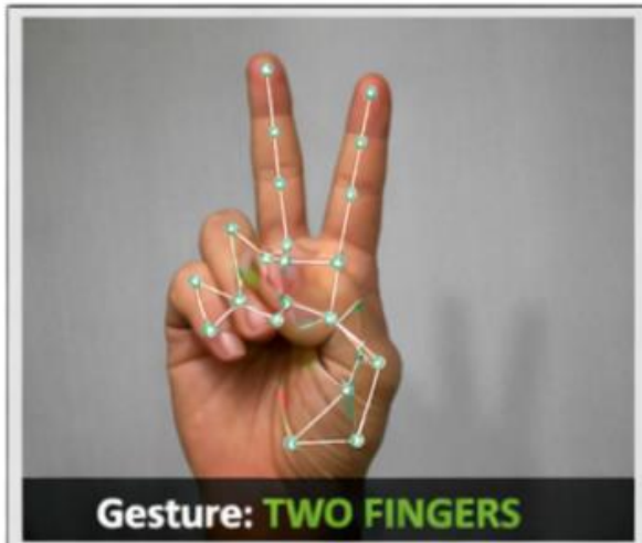
Fig. 2. Hand Gesture Recognition Using Mediapipe
