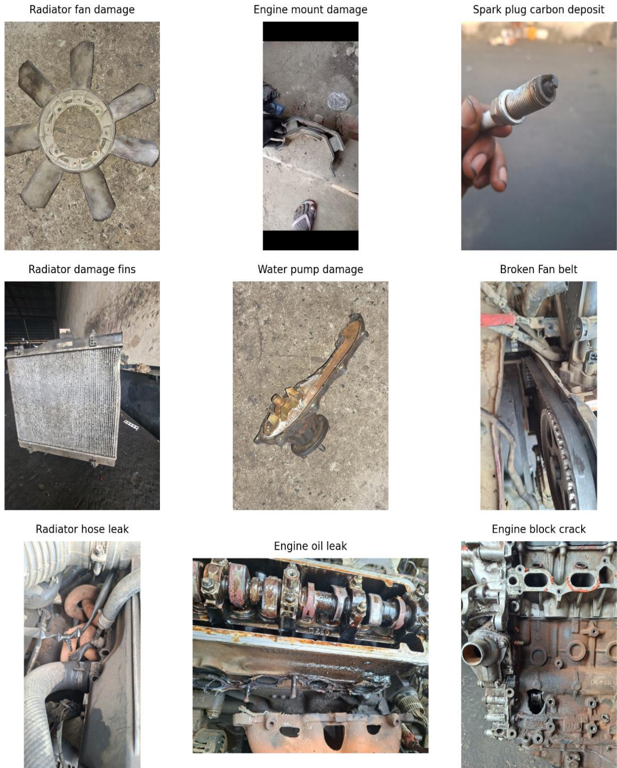
Figure 1: Sample automobile fault images collected from workshop environments including radiator fan damage, spark plug deposits, broken belts, radiator hose leakage, and engine block defects.
