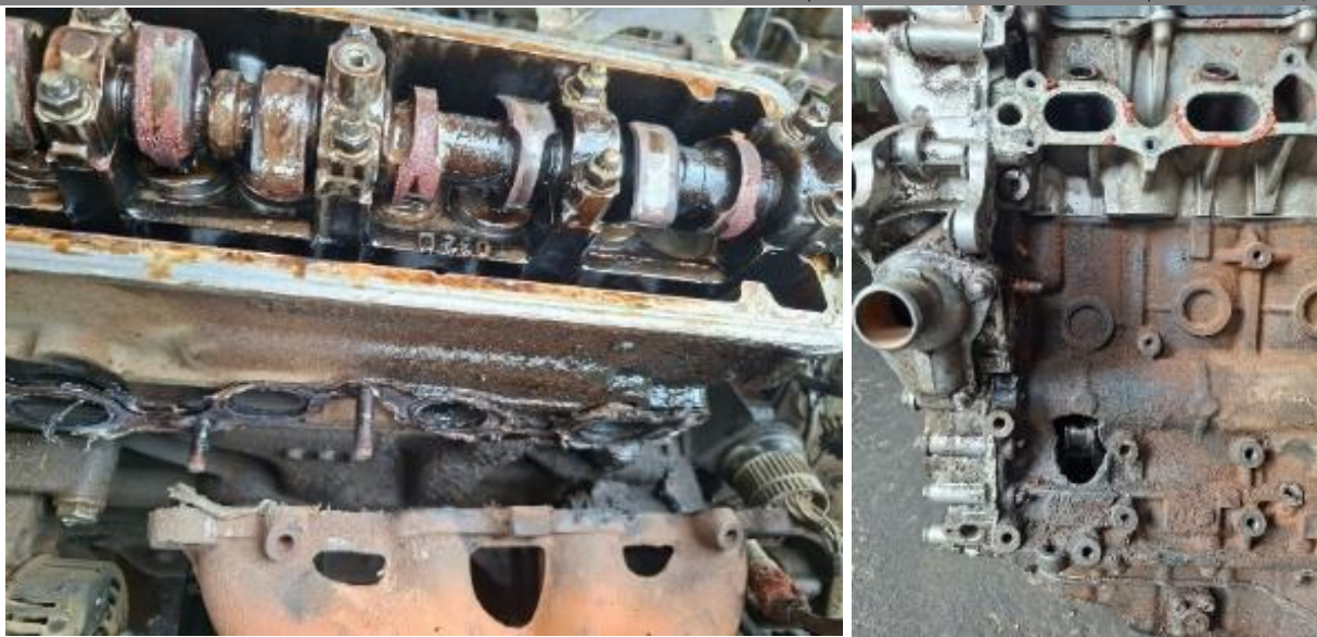
Figure 6: Engine oil leakage vs Engine block crack
