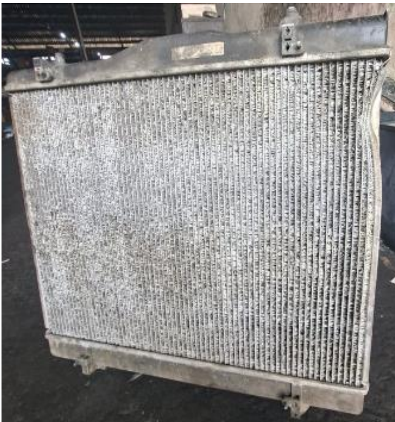
Figure 5: Structural deformation of radiator fins
