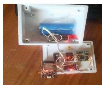
Fig. 3A. ESP 32-CAM on breadboard Fig. 3B. PIR connected to ESP 32-CAM Fig. 3C. System setup moved to plastic casing
