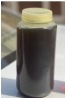
Figure 1. Contaminated hydraulic oil before the filtration process
