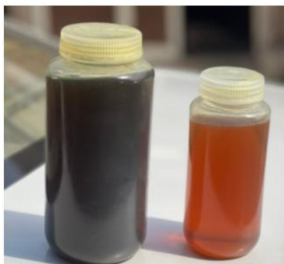
Figure 2. Hydraulic oil condition before and after filtration
