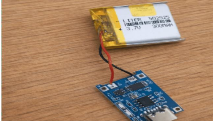
Fig. 5.3 Testing of 3.7V Li-Po battery
