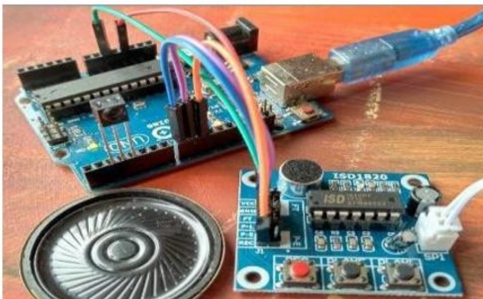
Fig. 5.2 Testing of Voice Module (ISD1820) with Speaker
