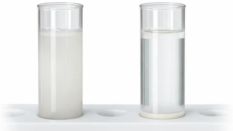
Fig 2 : Kaolin turbidity removal test demonstrating coagulation efficiency of Strychnos potatorum L seed polysaccharide at optimized dosage.
